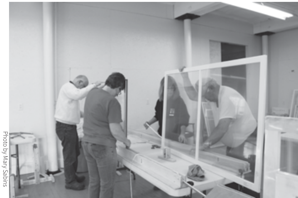
Volunteers apply foam to the outside perimeter of wooden inserts prepared at the Window Dressers Community Build workshop.
